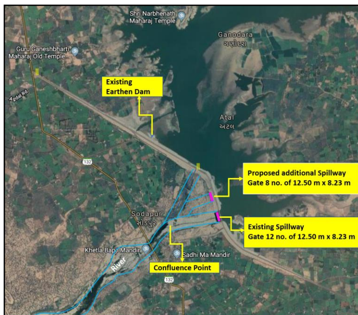
Figure 12. Proposed additional spillway
